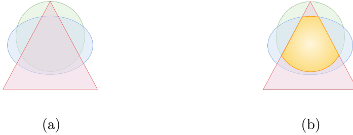
Figure 3.1: Visual representation of human and AI performances. On the left, the red triangle represents the ML model, the blue ellipse represents the human, and the green circle represents the ground truth. They are positioned in the solution space of a binary prediction problem. For every figure, positive answers are inside, and negative answers are outside, with the correct answers determined by the green circle. On the right we can see the yellow region representing the correct answers obtained by both the human and the AI model.
